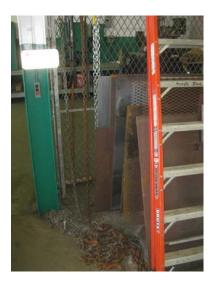
The two free standing gas cylinders in the garage building three need to be properly chained and secured. Recommendation 5-2016 (I)
